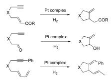
Using Pt<sup>II</sup> complexes and hydrogen, the reductive cyclizations of yne-enones, yne-aldehydes, and yne-dienes were conducted, which showed expanded reactivity of the Pt-alkyne complex with various electrophiles.
